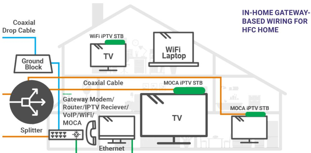
Wiring within the home could continue to be coaxial cable (using MOCA), or it could be Ethernet CAT-5 or CAT-6 twisted pairs. Other options include powerline or G.HN, or even no wires at all using Wi-Fi. This approach has been widely deployed by fiber-based broadband service providers. Wi-Fi is now the dominant approach to providing LAN connectivity within the home.
