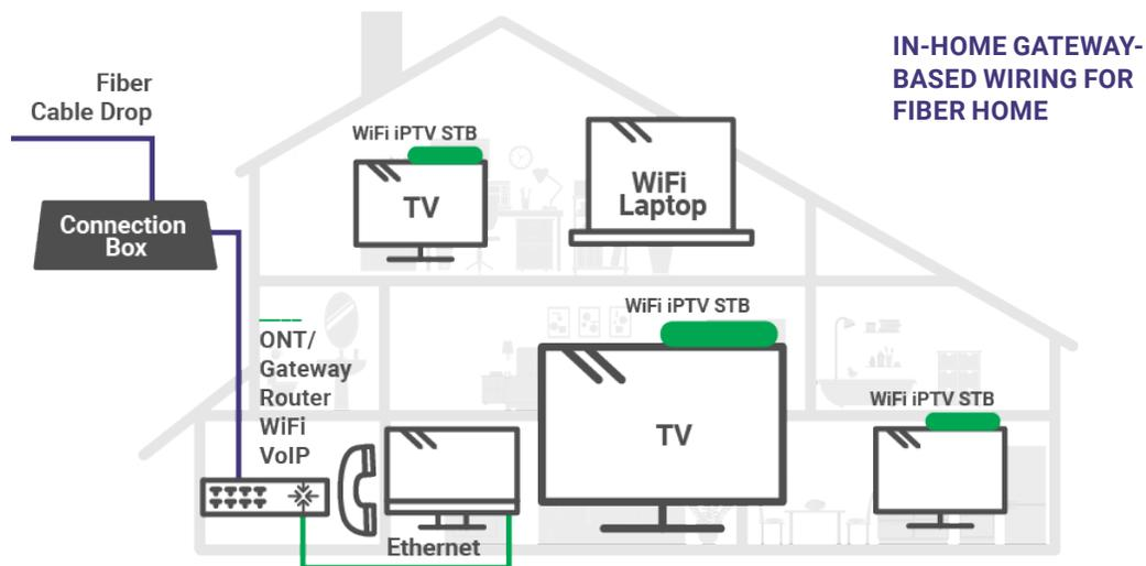
In a fiber home, the ONT terminates the outside plant optical signals, and from its associated router generates in-home signals for distribution via Wi-Fi, Ethernet, MOCA, or G.HN.
